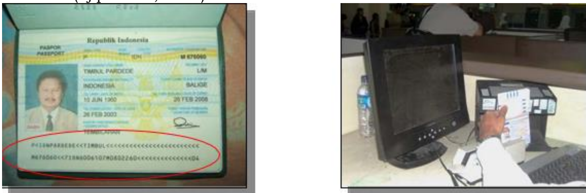
Figure 1. MRP passport with Machine Readable Zone characteristics at the bottom of the biographical page (left photo) and sweeping process (right photo).
